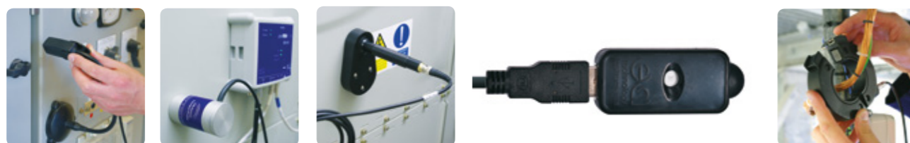
Options include (from left to right): ultrasonic microphone, contact ultrasonic sensor, plug-in TEV probe, temperature/humidity probe and Radio Frequency Current Transformer (RFCT)
