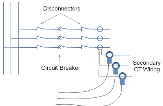
**Figure 2 Point for measuring the line currents**
