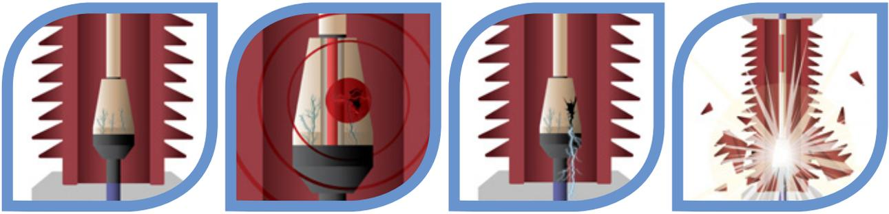
1. PD starts to erode insulation
